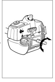
CAUTION! Contact your servicing dealer, if the idle speed setting cannot be adjusted so that the cutting attachment stops. Do not use the machine until it has been properly adjusted or repaired.
